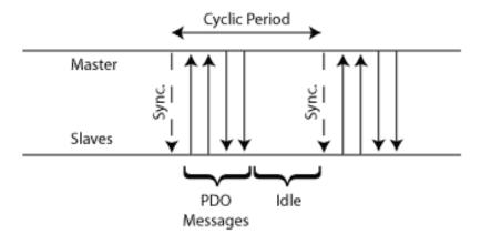
The advantage of this scheme is that it generates a predicable loading of data on the bus. The latency on transmitted data is predictable, but the latency is not the absolute minimum that can be achieved.
