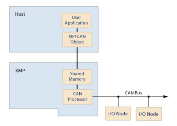
The XMP operates as a master node on the network with all the IO nodes being slaves. This arrangement implies that there may only be one XMP on any CAN Network.
