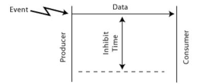
The advantage of this type of messaging is that short reaction times are attainable, but this is accomplished at the expense of variable network traffic, and the possibility of saturating the network. In many cases, the reaction time is not significant in relation to other time delays in the system (ex: the user's application or delays in task switching).
