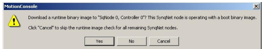
If the FPGA Runtime has not been previously installed the following message is displayed.
