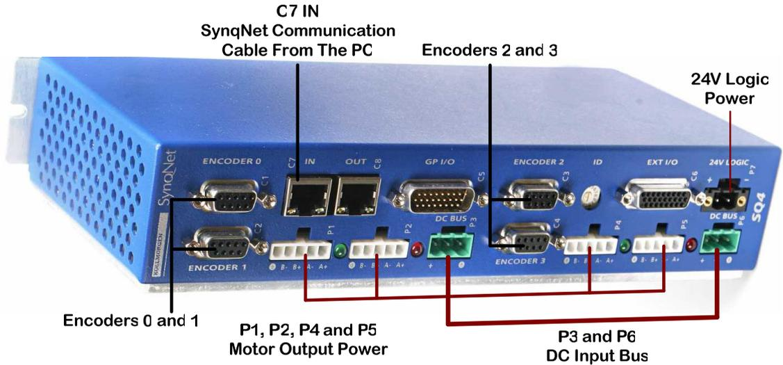
Figure 1: Front Cable Connection Panel
