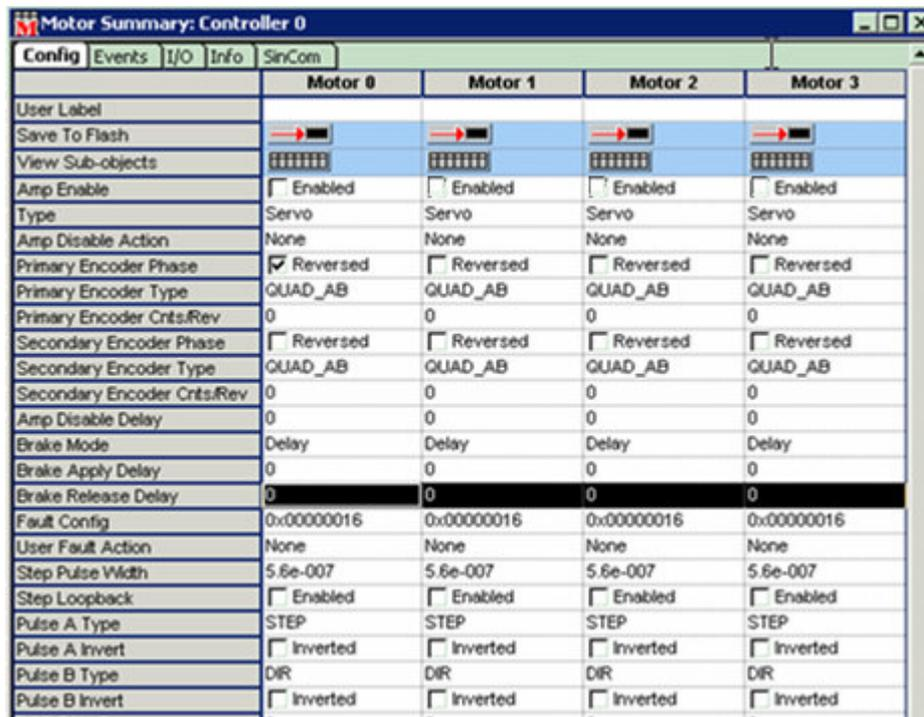
5. Set the **Type** to **Servo** for all four axes.
