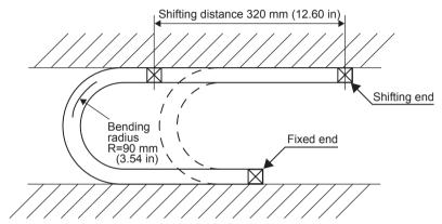
Note: 1. The life of flexible cable differs largely depending on the amount of mechanical shocks, mounting to the cable, and fixing methods. The life of flexible cable is limited under the specified conditions.
