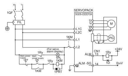
1QF: Molded-case circuit breaker1Ry: RelayFIL: Noise filter1PL: Indicator lamp1KM: Magnetic contactor1PRT: Surge protector1D: Flywheel diode
