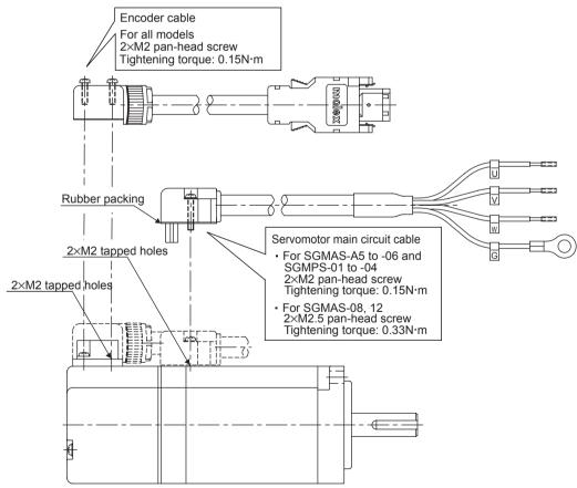
Note: Do not remove the rubber packing on the servomotor-end cable connector. Mount the connector so that the rubber packing is seated properly.
