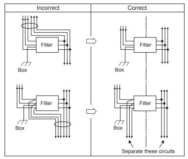
Separate the noise filter ground wire from the output lines.
