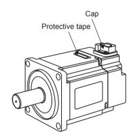
2. Mount the cable connector on the servomotor and fix it with screws as shown in the figure below.
