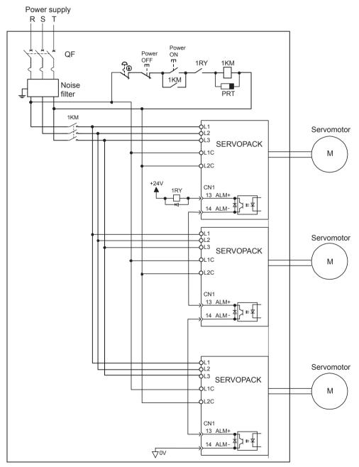
Note: Wire the system so that the power supply's phase-S is the ground.
